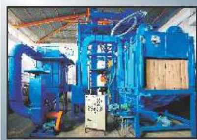
Airless Tunnel Type 10 Wheel Blasting M/c for 'I' Section Cleaning
