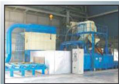
Airless Tunnel Type 4 Wheel Blasting M/c with Pre Heating Chamber for Plate Cleaning
