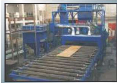
Airless Tunnel Type 6 Wheel Blasting M/c for Plate Cleaning
