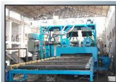
Airless Tunnel Type 4 Wheel Blasting M/c for Plate Cleaning
